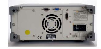
The V60 Series rear panel layout includes three standard remote interfaces: A fully programmable RS232 port, a PLC Interface port and a High Voltage Scanner control port. Available options include GPIB and rear terminal outputs.
